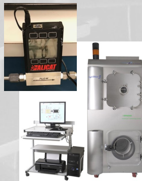
LYOSTAR™ 3 Freeze-Dryer with controlled nucleation and mass flow meter
