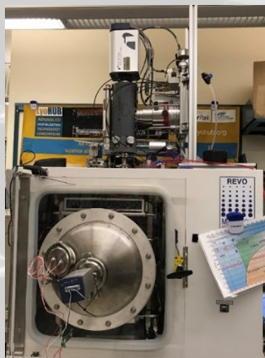
Figure 1. Residual gas analyzer (RGA) from INFICON and its components.
