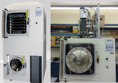
REVO lyophilizer with controlled nucleation and in-situ mass spectrometer.
