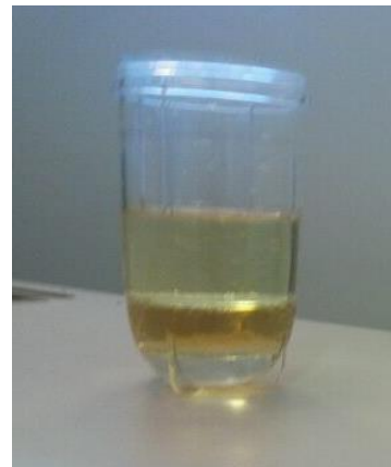
Figure 5. Separation of ingredients: Oil (top), Vinegar and water (middle), corn syrup (bottom).
