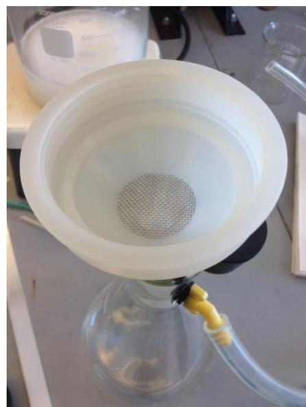
**Figure 2. Funnel and screen setup for pouring into flask.**
