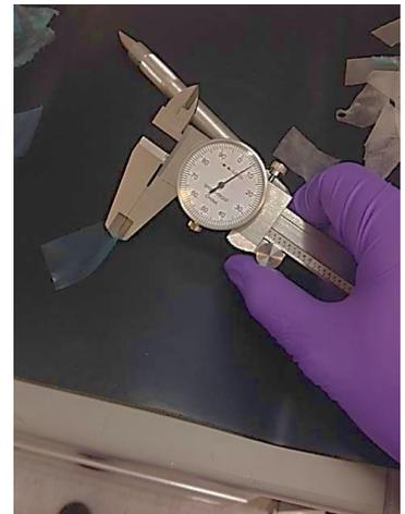
**Figure 6. How to use calipers**
