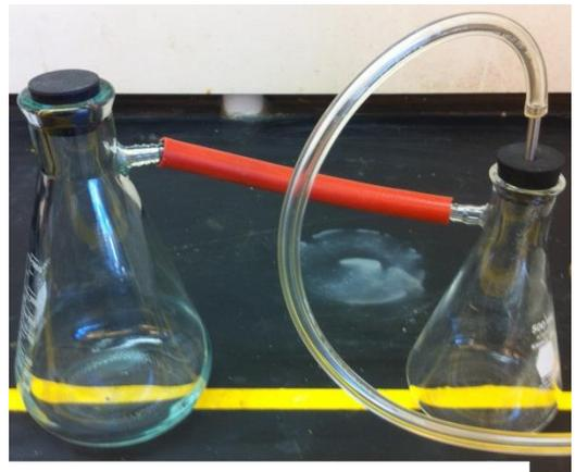
**Figure 3. The setup that should be used when using the vacuum.**
