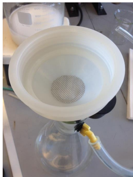
Figure 1. Funnel and screen setup for pouring into flask.
