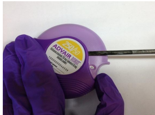
Figure 2: Removal of outer shell
