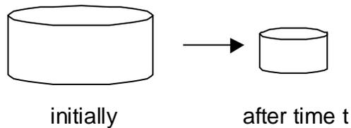
Chemical Engineers who work on drug formulations are concerned with obtaining the desired dissolution rate. We must be able to measure the drug dissolution rate, and we must also be able to describe the drug dissolution using a mathematical model. These equations should match the experimental data.
