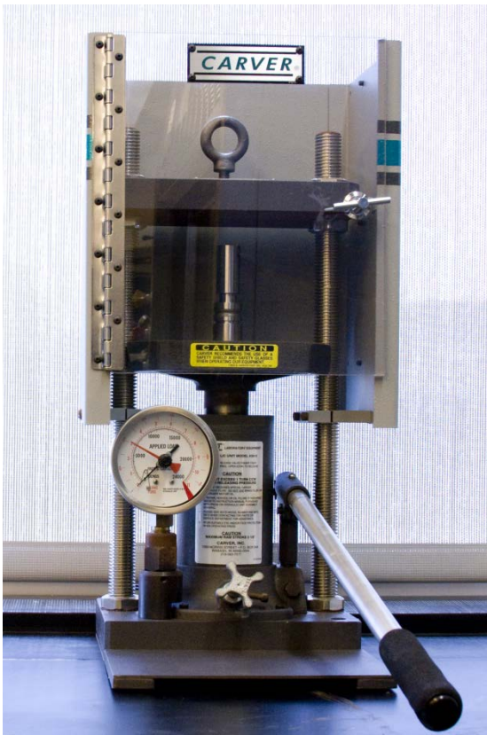
Figure 8. Punches and die on the tablet press prior to compression.
