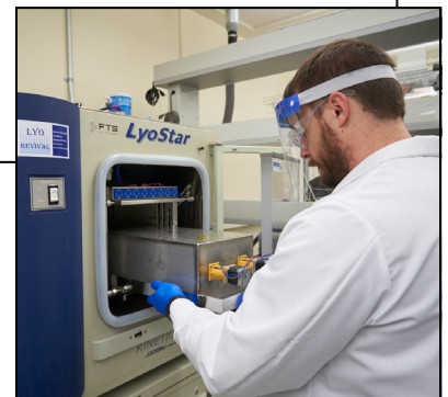
Figure 1: Random field radio frequency lyophilization experimental setup (left) and block diagram (right).
