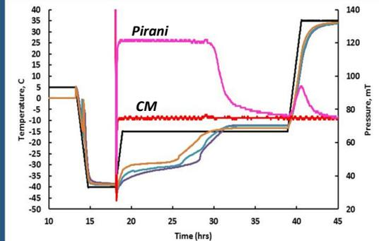
Use capacitance manometer with temperature-controlled sensing head for pressure measurement and control in a pharmaceutical freeze dryer.
