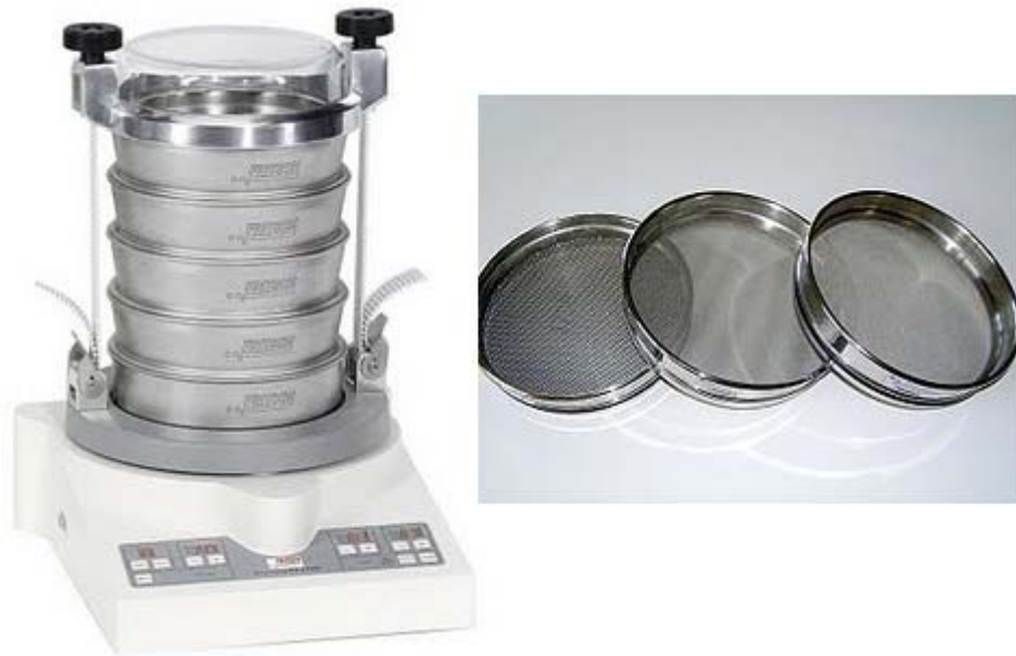
Figure 1: Example image of sieve shaker equipment and wire cloth sieves
