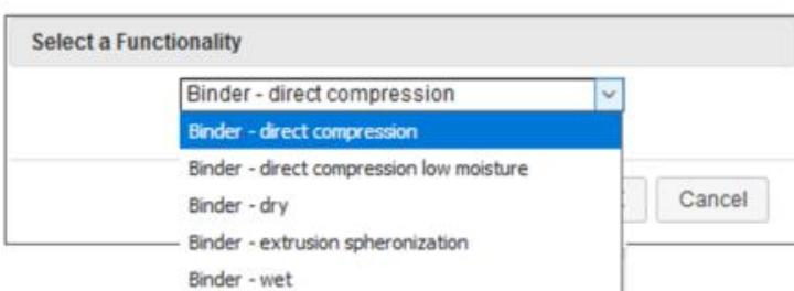
We select *Binder – direct compression* and click on OK. The functionality button turns a bright blue, and manufacturing method can now be selected. We continue to select options using the “top path” for the tool, and click on the Manufacturing Method button.
