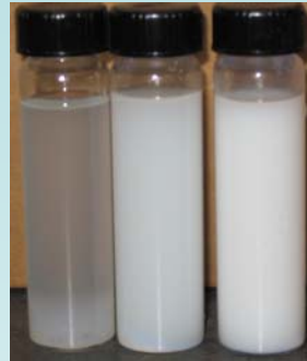
Ultrasonicing for 1 min. (a) DCM; (b) DCM 50 vol% in acetone; (c) Acetone
